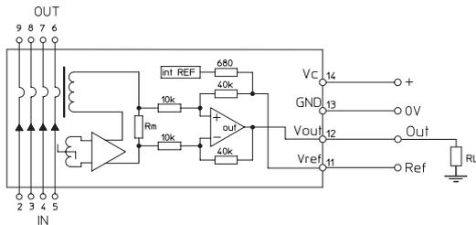
Figure 31: Test connection
